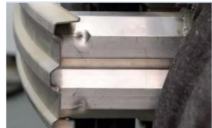
Buick LaCrosse Roll Formed Bumper/Extruded C.Box
