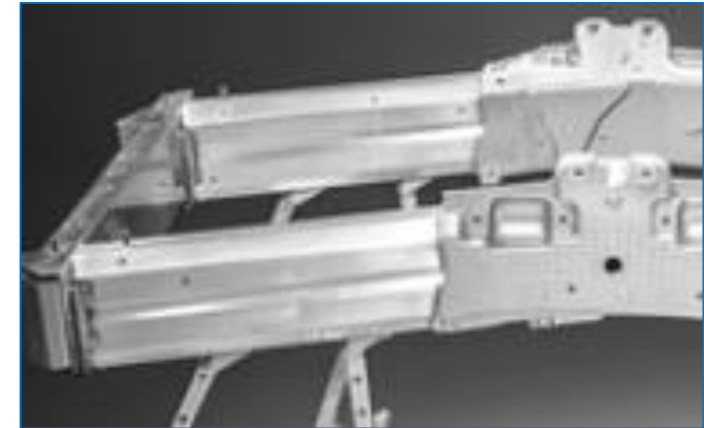
Corvette C7 Crash Box In Extruded 7xxx
