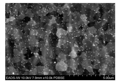
Grain sizes varies from 5 – 20  $\mu$ m (equi-axed) & 25 - 100  $\mu$ m (elongated) and 500 nm – 2  $\mu$ m in the very fine equi-axed region
