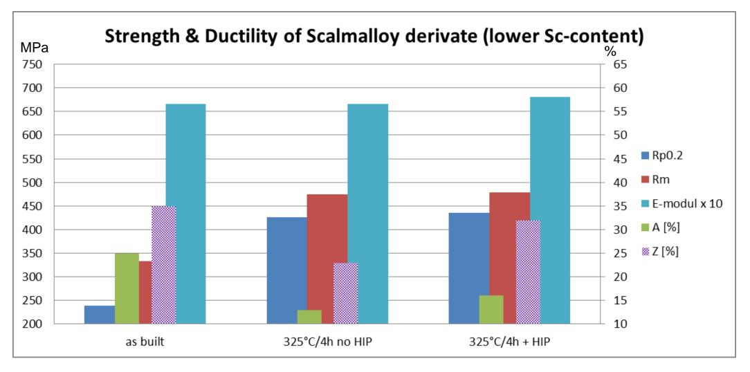
→ Evolution of Scalmalloy<sup>®</sup> material performance parameter (reasonable process parameter) due to post built-up heat treatment (incl. HIP) with respect to UTS / YS / A / Z & Y-M
