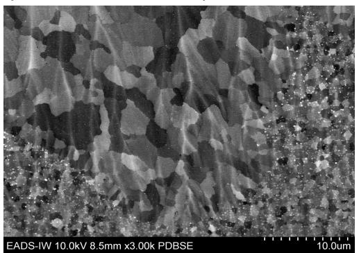
Bi-modal micro-structure with equi-axed (cast) grains in z-build-up direction & equi-axed + elongated grains in the x-y plain
