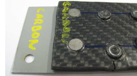
Semi-tubular self piercing rivet: Damage of the fibre-reinforced material by squeeze force and process fluctuations Source: Magna
