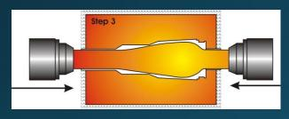
The positioning of material under hot gas pressure with material supply pushed in from both ends defines the final (local) tube thickness
