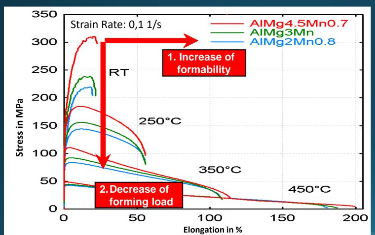
Effects of Temperature and Strain Rate on Strength and Formability:
