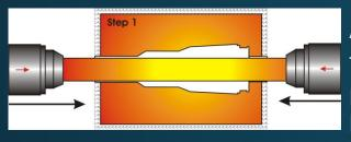
A tube is heated up to an temperature profile, then is placed into an adequately heated die and sealed at both ends.
