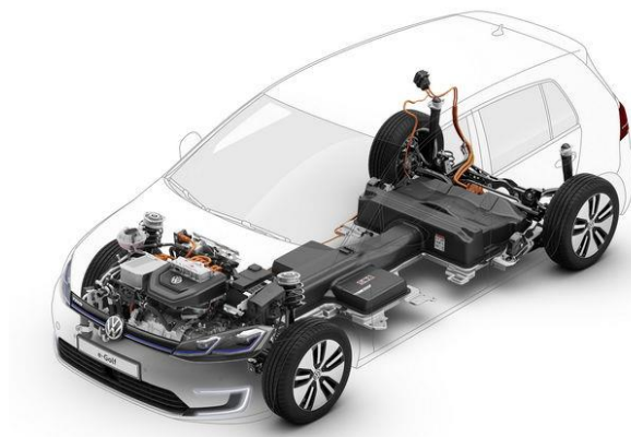
e-Golf's High-Voltage Battery System
