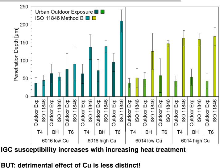
$\rightarrow$  Cu less critical for in-service conditions than usually assessed using immersion tests?
