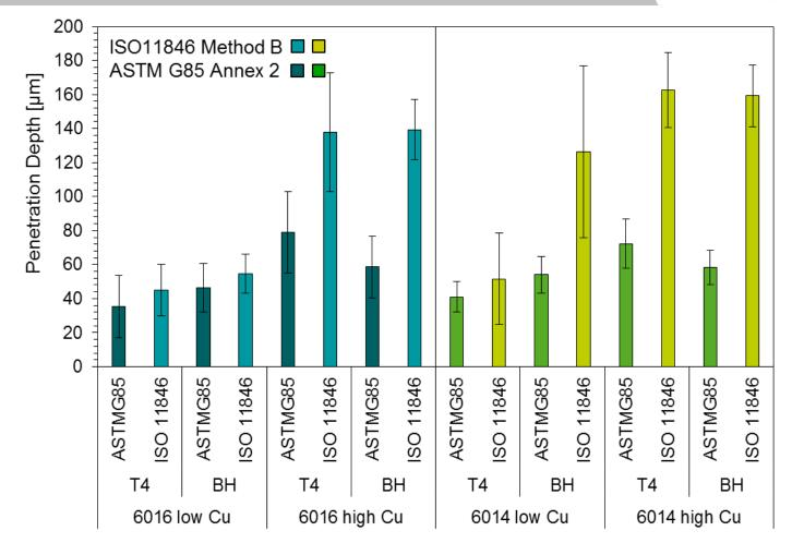
Influence of heat treatment and Cu-content seems to be rather low (at least when compared with immersion tests)
