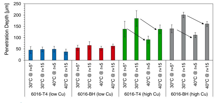
The solution temperature can significantly influence the test results!
