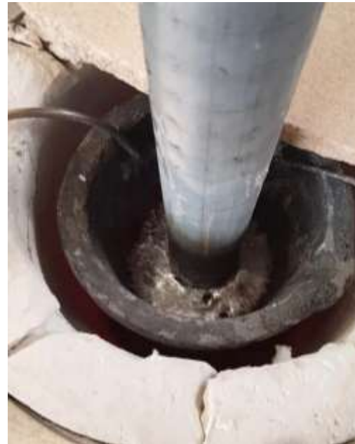
(a) SiAlON sonotrode in the melt, (b) mold design (c) cast specimen
