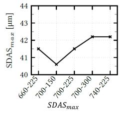
■ No significant impact → Feeder patch and wall thickness impact is more dominant than temperature
