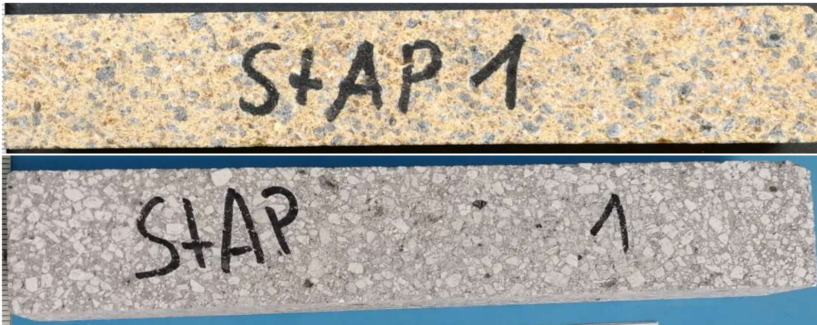
REFRAL S 62, cross section, Lab. test: 100% H 2 , 1400°C, before and after testing
