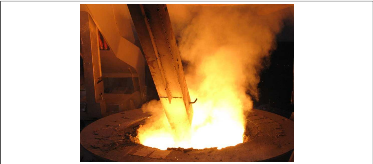
Fig. 7: Melting down ferrosilicon fines
