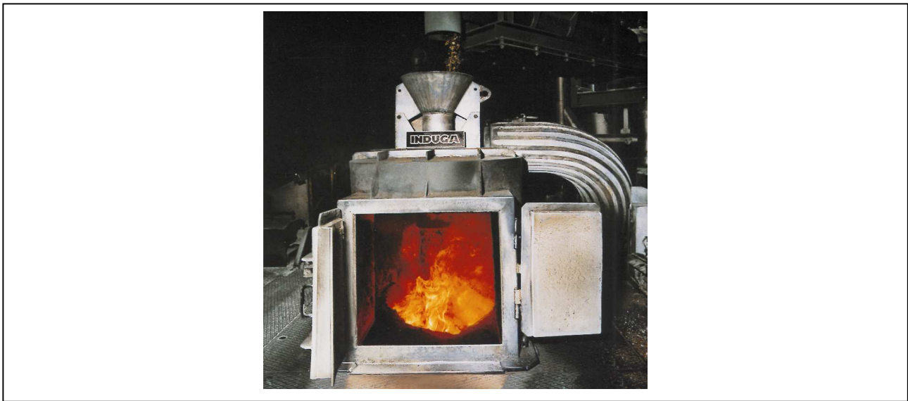
Fig. 6: Wet brass chip melting furnace
